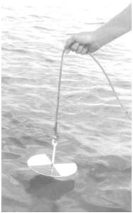
(Secchi Disk being lowered into the water)
