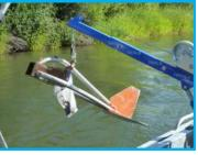
A Helly-Smith sampler was used to measure bedload. The bag collects the sediment sample.
