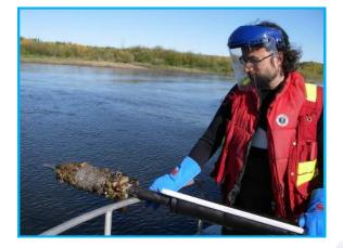
Physical Monitoring of the Gravel Pads: Andre Zimmerman from NHC Consulting pours liquid nitrogen into a metal pipe. The freeze core substrate sample is obtained by pounding the pipe through the gravel pad, 2011.
