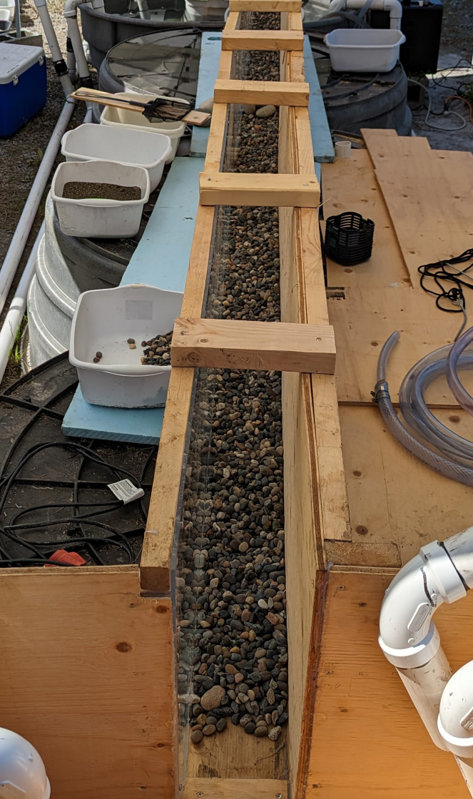
LEFT and ABOVE: Overview and side view of the flume that was constructed to test larval sturgeon settlement at differing flow velocities. BELOW: Screenshot from video showing larval sturgeon dispersing down the flume in moving water. Photo provided by Angie Coulter.
