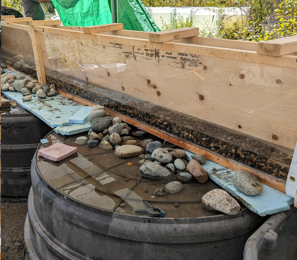
LEFT and ABOVE: Overview and side view of the flume that was constructed to test larval sturgeon settlement at differing flow velocities. BELOW: Screenshot from video showing larval sturgeon dispersing down the flume in moving water. Photo provided by Angie Coulter.
