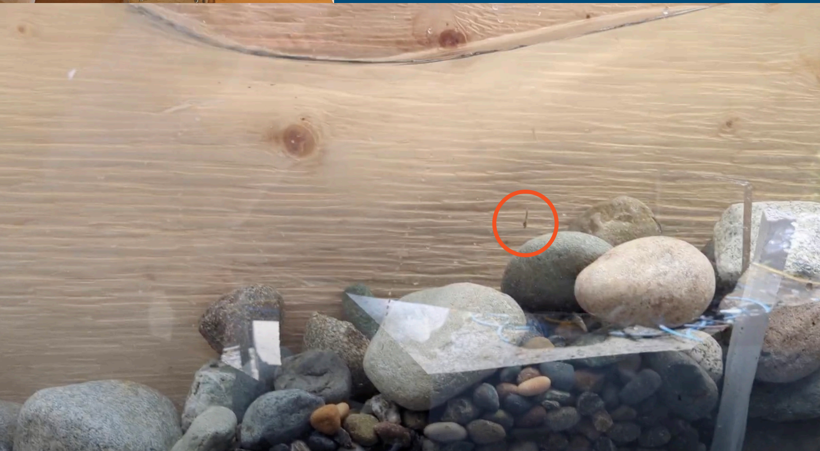
LEFT and ABOVE: Overview and side view of the flume that was constructed to test larval sturgeon settlement at differing flow velocities. BELOW: Screenshot from video showing larval sturgeon dispersing down the flume in moving water. Photo provided by Angie Coulter.
