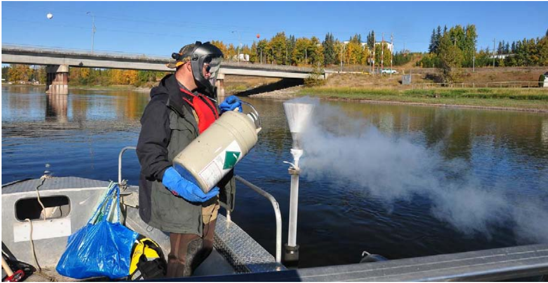
Photo 1: Liquid nitrogen being poured into the funnel that leads into a 20 mm diameter pipe that has an outlet 10-30 cm above the bottom of the core.
