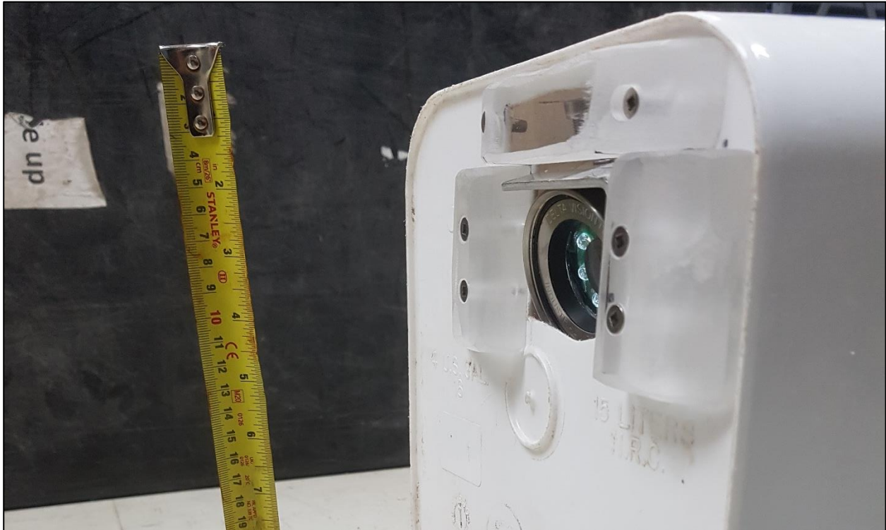
Photo 2.4 Plastic housing for the underwater camera installed to minimize risk of fouling due to debris accumulation.
