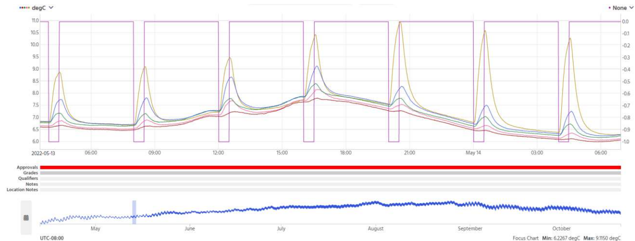
Figure 4.2 All five sensors on Grid 1377 showing a response to heating after 2022-05-12; Sensor 1 shown in blue, Sensor 2 shown in dark red, Sensor 3 shown in green, Sensor 4 shown in pink, Sensor 5 shown in dark yellow, and Heater shown in purple (0 = OFF, -1 = ON).
