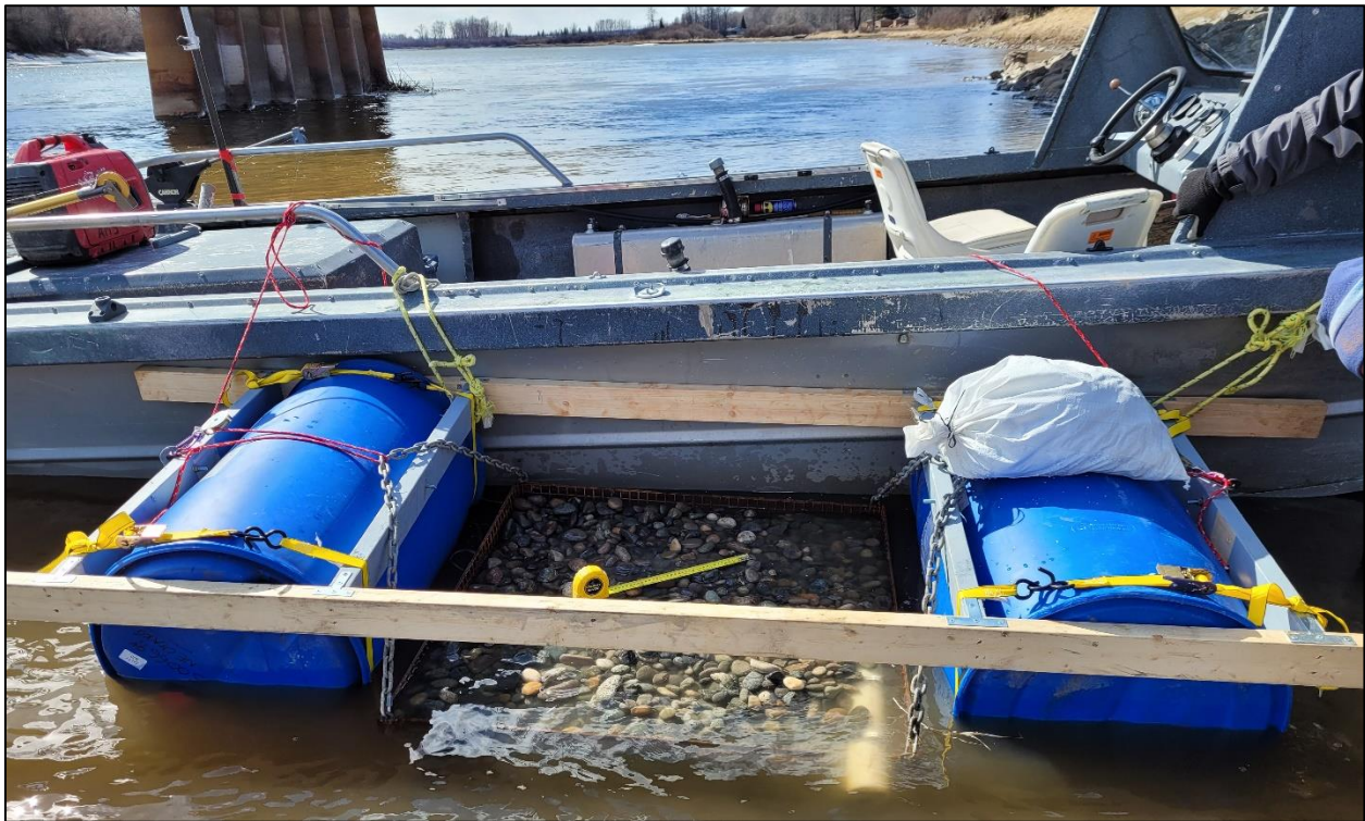
Photo 3.5 Pontoon system used to lower the sensor arrays onto the riverbed.
