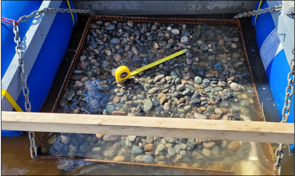
Photo 2.3 Sensor array covered with clean gravel prior to deployment.
