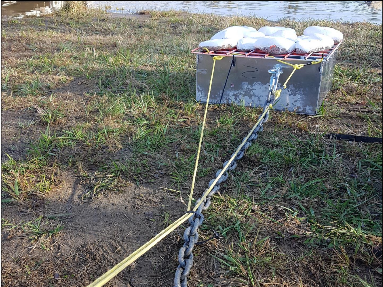
Photo 2.6 Front-view of the sediment trap showing the anchor chain attachment and drawstrings used to close the sample bag prior to retrieval.
