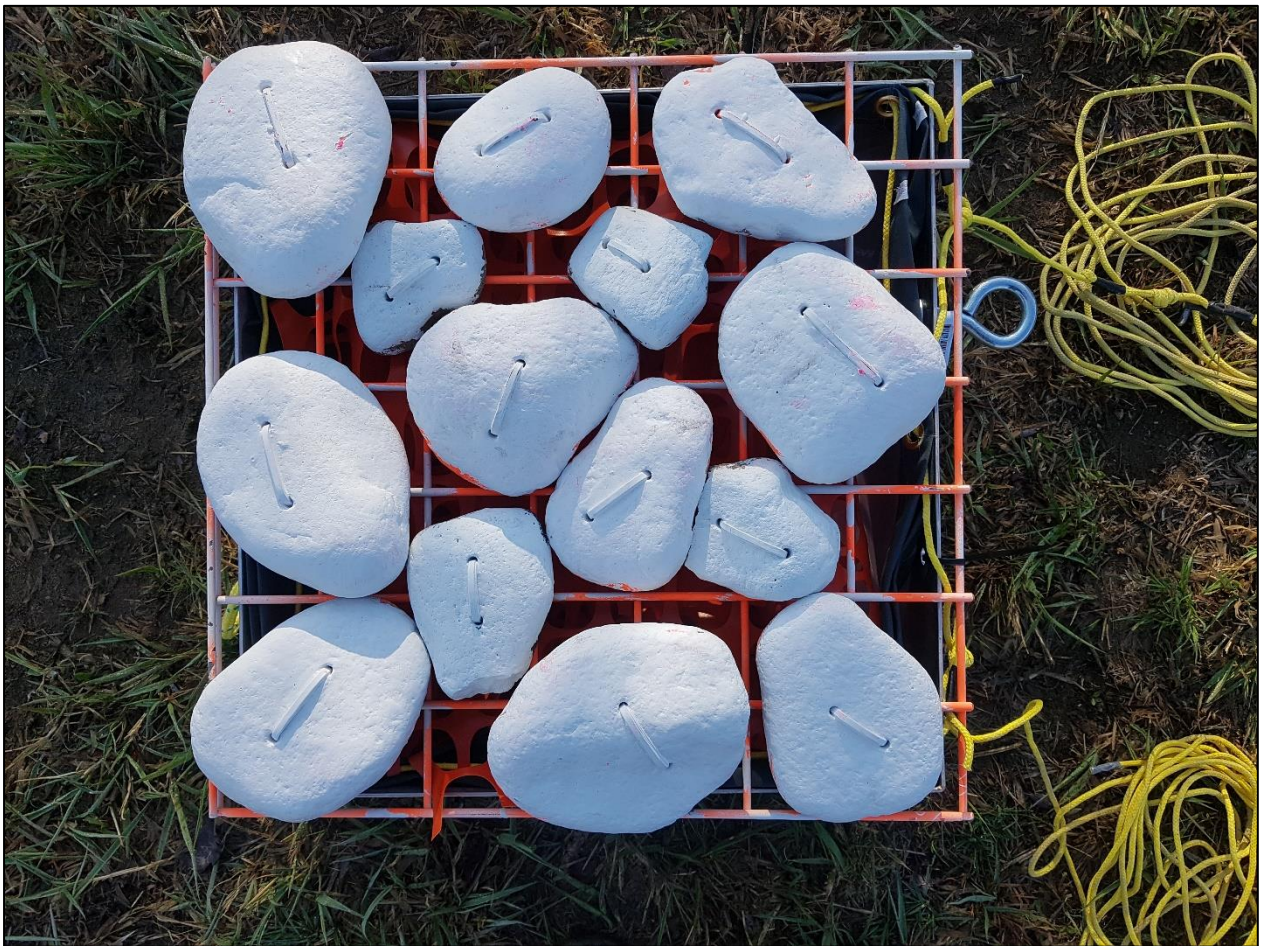
Photo 2.5 Overhead view of sediment trap showing hinged lid with cobbles, 125 micron mesh sampling bag and snow fencing to prevent scour and loss of collected sediment.
