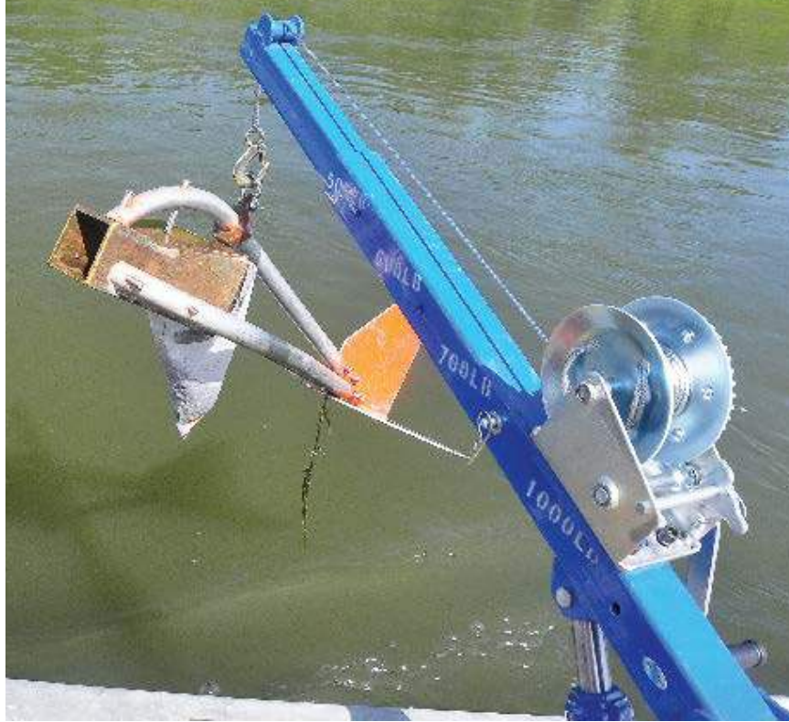
Figure 2 Photo showing the Helley-Smith sampler and crane mount that were used.
