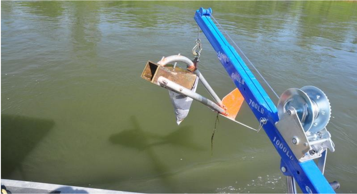
Figure 2: An example of the bedload captured
