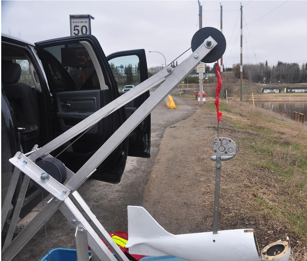
Figure 3: Suspended sediment sampler with nozzle installed and mounting bar installed
