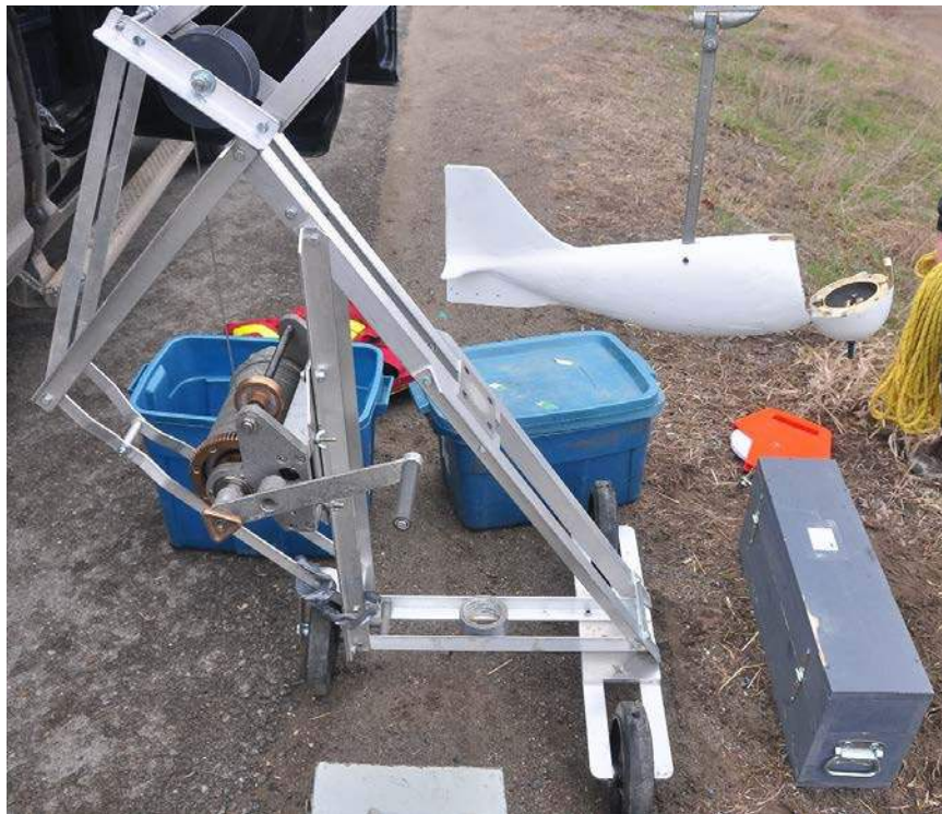
Figure 3 Bridge Crane with suspended sediment sampler and B-reel.
