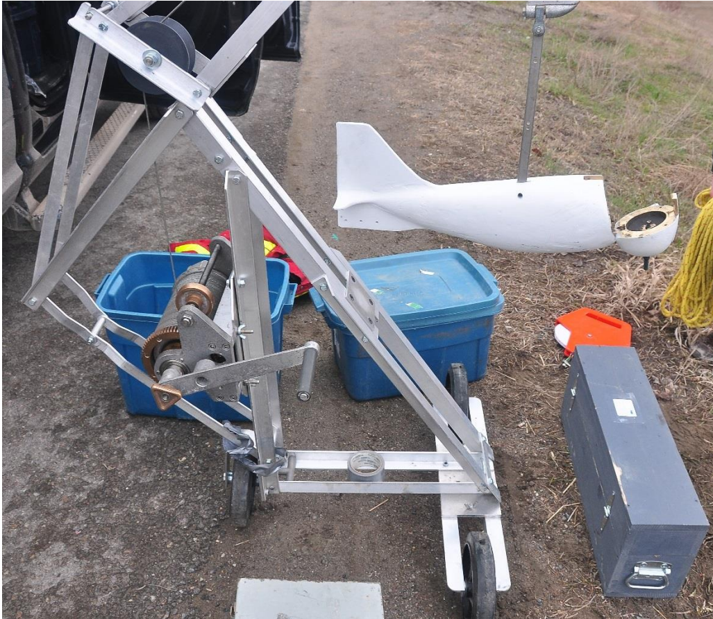
Figure 1: Bridge Crane with suspended sediment sampler and B-reel
