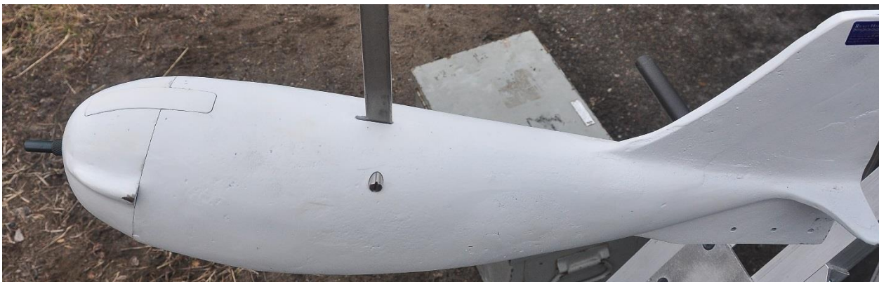
Figure 3: Suspended sediment sampler with nozzle installed and mounting bar installed
