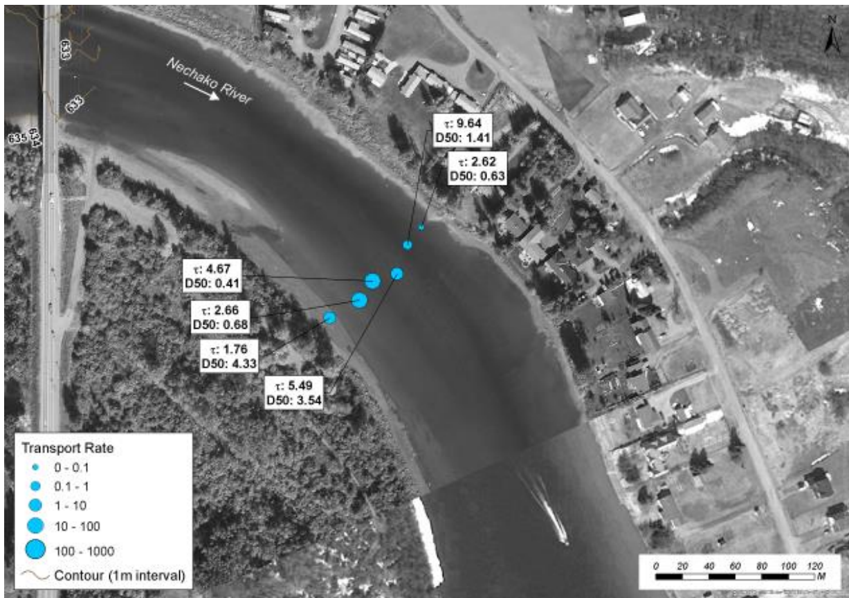
Figure 10: Overview of the sampling sites for the Lower Site. Shear stress (Pa) and D_{50} (mm) are given for each station. Transport rate (g/m/s) is represented by the size of the circle.
