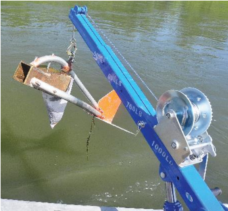
Figure 3: Photo showing the HellySmith sampler and crane mount that were used.
