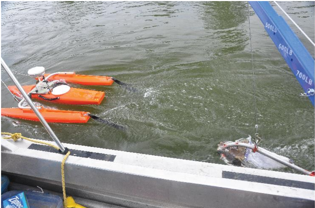
Figure 4: GPS mounted above ADCP that was used to determine velocity and moving bottom conditions.
