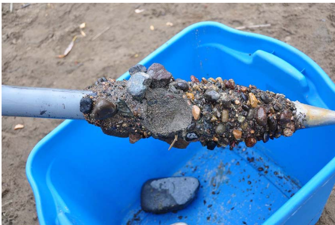
Figure 6: Photo of Core 5 from the lower site. Fine gravel and coarse sand fill the interstitial spaces around the larger placed stones. The substrate below the larger stones is the native material. The native material is composed of clast supported gravels with a sand matrix.
