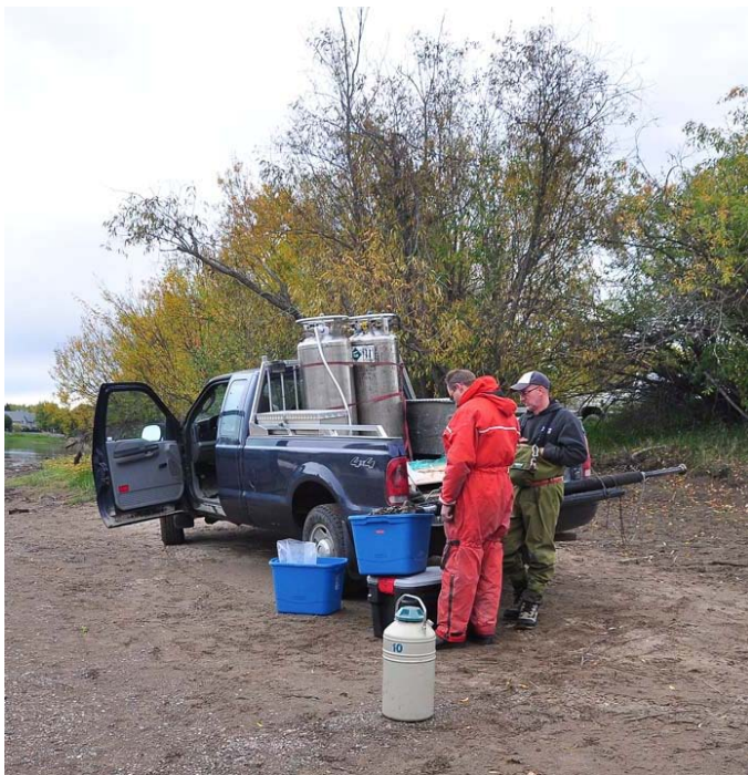
Figure 5: Two 160 Litre dewars of liquid nitrogen are in the back of the truck and a 10 L dewar used to pour liquid nitrogen into the cores is visible in the foreground.
