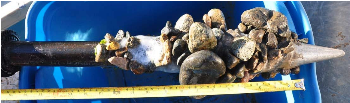
Figure 10: A photo of Core 9 showing the ice filled pore spaces. The fine sediment that does occur would have likely moved as suspended sediment. The placed pad was evidently quite thick at this location.
