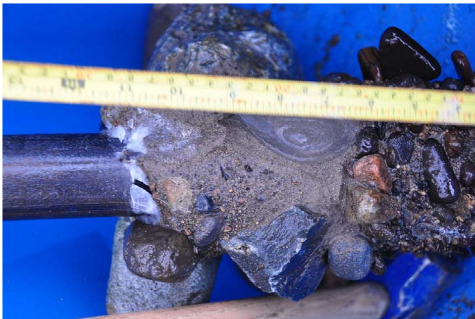
Figure 7: Core 3 from the lower site. The abrupt transition at 26 cm represents the transition from the native material (to the right) to the placed material. The fine matrix material that has filled in the interstitial spaces between the placed sediment grades from medium to fine sand at the bottom of the placed material to coarse sand at the top. The vertical coarsening likely represents the progressive infilling of the substrate as coarser material began to move downstream over the pad and infill the pores.
