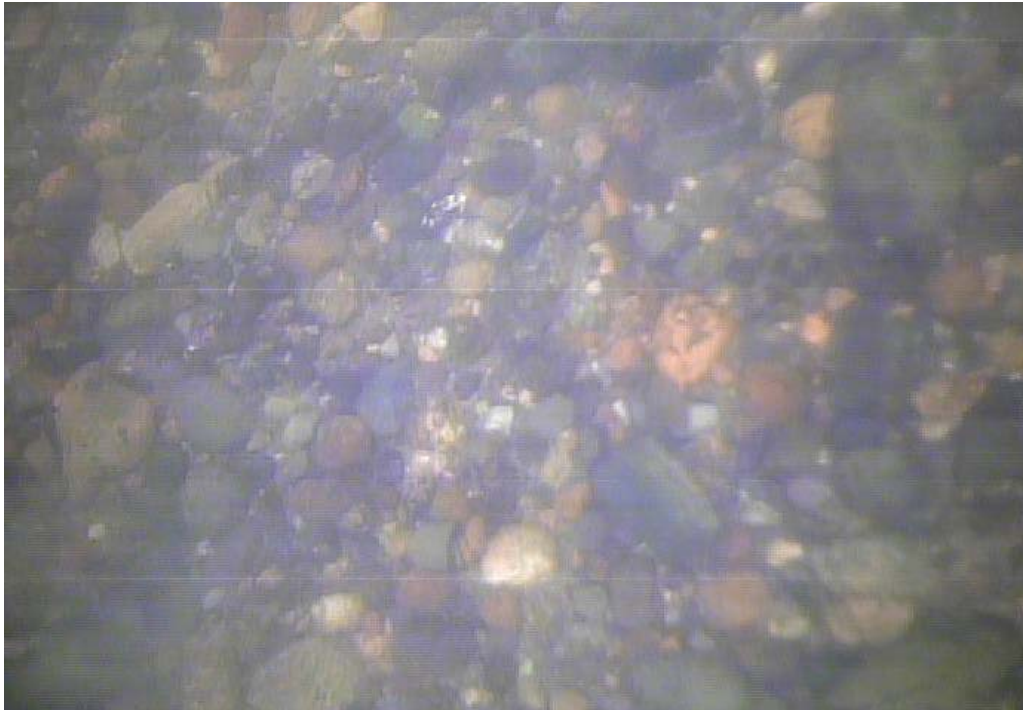
Photo 8: Image of native substrate that does not have a sand drape over the gravel. Photo taken 45 m upstream of lower pad in center of channel.
