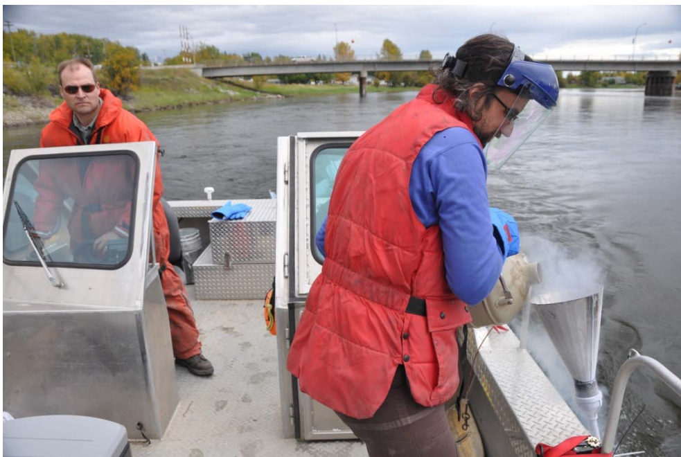
Figure 3: Liquid nitrogen being poured into the funnel that leads into a 20 mm diameter pipe that has an outlet 10-30 cm below the bottom of the core.
